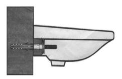
Place the basin in position against the wall, locating the fixing bolts through the holes in the rear of the basin. Push a plastic washer followed by a metal washer onto each fixing bolt.
