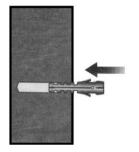
Push a dry wall anchor into each hole.
