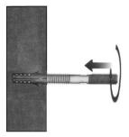
Screw a fixing bolt into each fixing plug using an 8mm spanner until the spanner contacts the wall.
