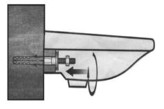
Screw a metal nut onto each fixing bolt to secure the basin. **Caution**: Do not over tighten as this may damage the ceramic.
